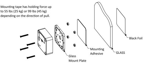
18-GLASS-LATCH-KIT Set includes mounting plate, double-sided adhesive tape, black foil, and 4 screws.
