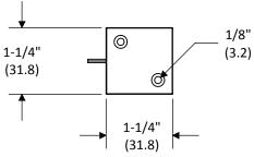
Spacer plate prevents wires from being crushed against the mounting
