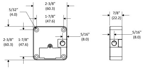
18-FPS-SOLO-RELAY Solo-Relay: 125 kHz Access Control Unit
